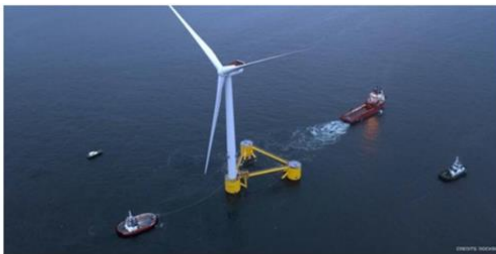
Figure 19. WindFloat Wind Turbine transport to Viana do Castelo 52
